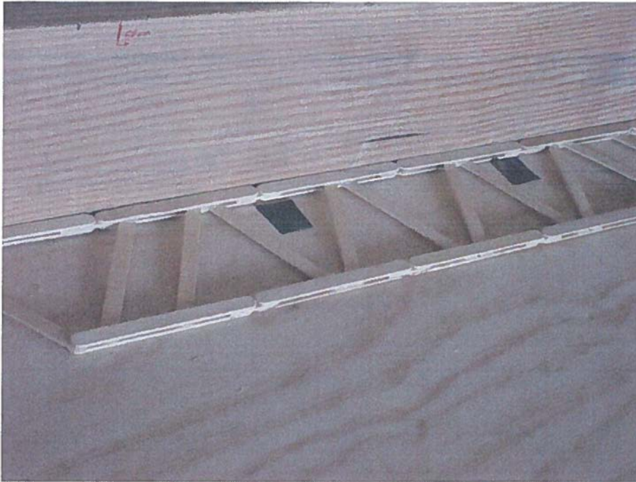
Photo 10. Add a 2"d layer of sticks to the beams for extra strength. Trim off any excess stick ends.
