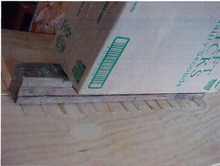
Photo 6. When you are done gluing the sticks, place a heavy weight onto the deck for several hours until the glue dries.
