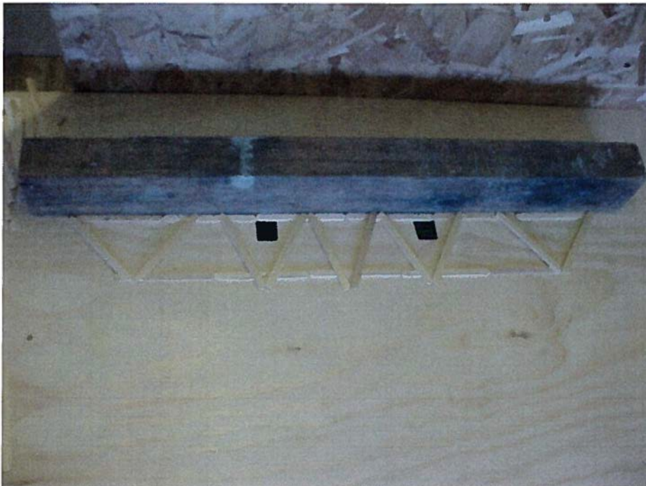
Photo 7. We begin by loosely placing the sticks in the desired pattern on our work surface. (The truss is shown upside down in the photo.) A symmetrical pattern looks good. Use your imagination here. Any pattern of truss will work. Try to use triangles within your trusses. Triangles are strong structural components.
