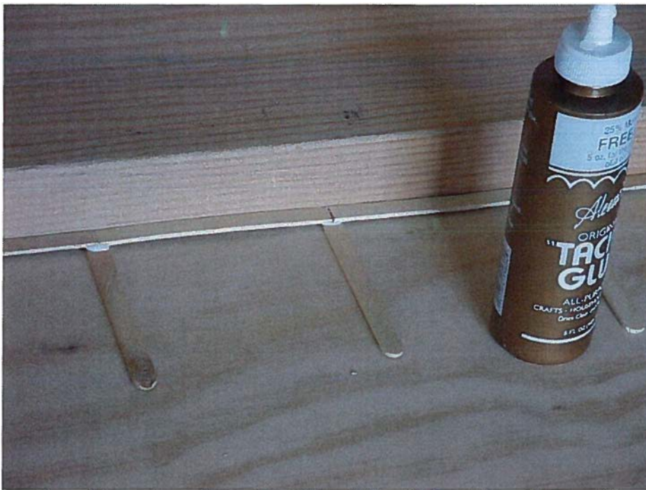
Photo 4. Next, glue the sticks which form the bridge deck to the ribs. Place the first row of sticks tightly against the straight edge (the 2" x 4" lumber), being careful not to glue the sticks to the straight edge. This ensures that the deck will be straight.
